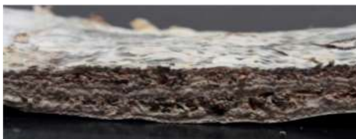
Figure 3. Section of a mycelium sheet [7]
