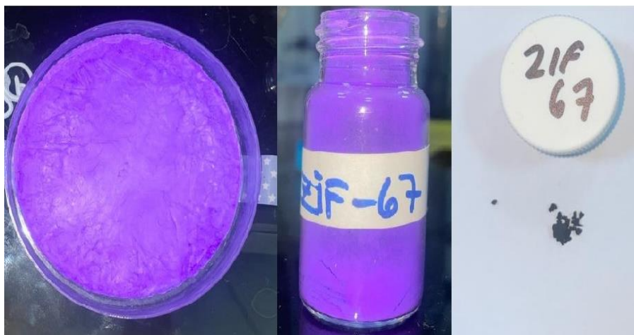
Figure 1. ZIF-67, from left to right after synthesis, powder form, and after pyrolysis stages.
